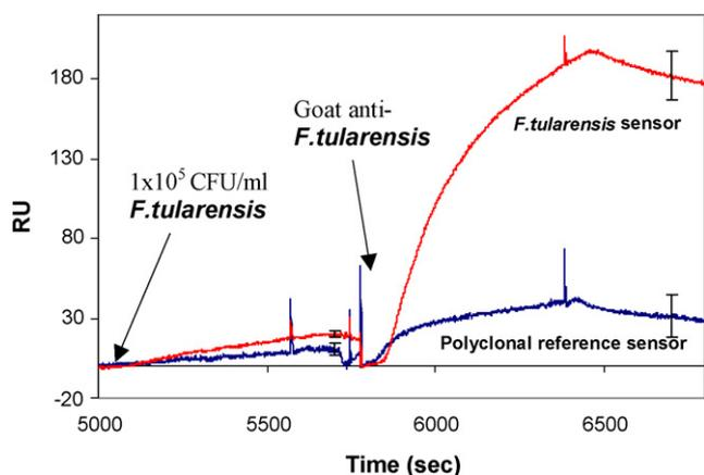
Fig. 5. Detection of  $1 \times 10^5$  CFU/ml *F. tularensis*. The average response of three sensor with goat anti-*F. tularensis* surfaces is compared to the average of two channels with normal goat serum surfaces. Error bars indicating the deviation between channels are shown every 900 s. Arrows indicate when sample was injected and when the amplifier was injected into the SPIRIT system.
