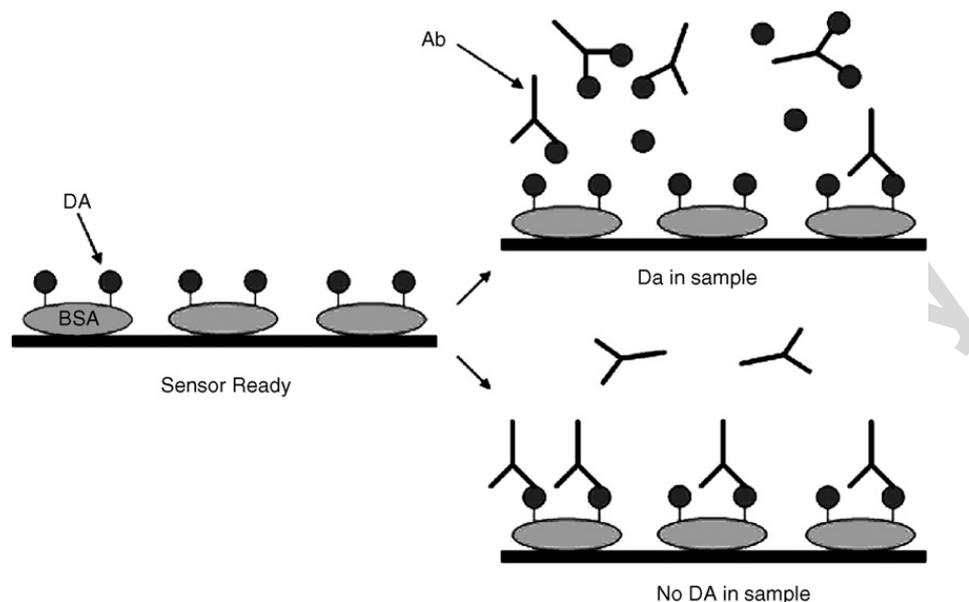
Fig. 5. Competition detection of a small molecule using SPR. A schematic of the sensor surface shows the DA-conjugated BSA on the surface of a sensor in the 'sensor ready' state. The quantity of antibodies that binds to the surface during exposure to sample is inversely correlated to the amount of DA in the sample.
