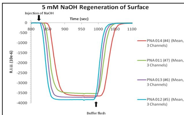
**Fig. 4:** Regeneration of probe layer with 5 mM NaOH. Return of RIU to pre-experimental baseline level indicates successful removal of bound material.
