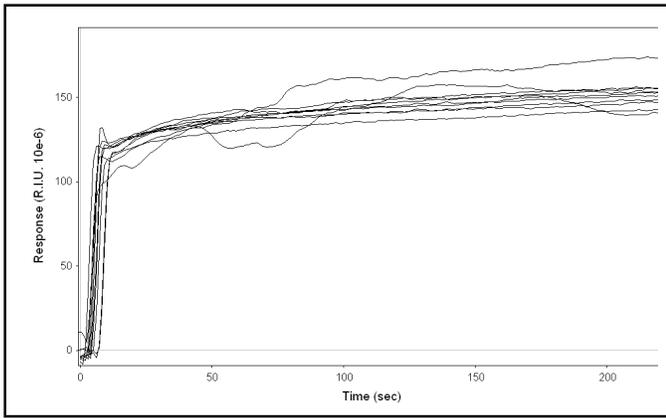
**Fig. 5:** SPR detection of *Alexandrium fundyense* oligonucleotide by PNA probe 008, with the reference channel subtracted. A total of 40 experimental cycles of introducing oligonucleotide complimentary to the PNA probe and then regenerating the surface by removal of bound material with 5 mM NaOH were performed before seeing a 10% loss of R.I.U.
