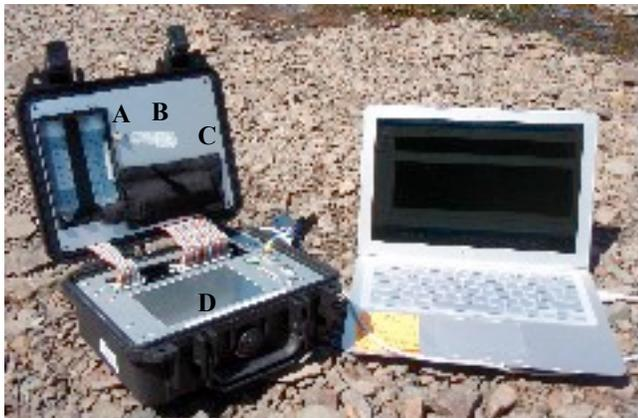
**Fig. 2:** Custom-built SPR instrument developed at the University of Washington (SPIRIT, sold by Seattle Sensor Systems, Inc.). A=Buffer tube, B=Syringe in sample injection port, C=24-channel sensor bank, D=touch screen controls. Data outputs to directly to a PC software program that allows for real-time monitoring of the SPR response.
