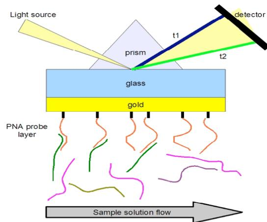
**Fig. 1:** SPR operation with PNA probe layer on gold surface. Binding of target molecules causes a change in refractive index.
