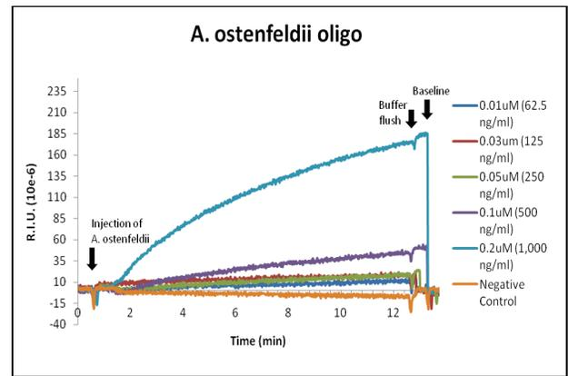
**Fig. 6:** SPR detection of *Alexandrium ostenfeldii* oligonucleotide by PNA 013 at multiple concentrations. This method can still detect quantities of this oligonucleotide down to concentrations of 0.01 $\mu$ M, though quantities below 0.05 $\mu$ M were undistinguishable from lower concentrations. No detection of binding with negative control PNA probe.
